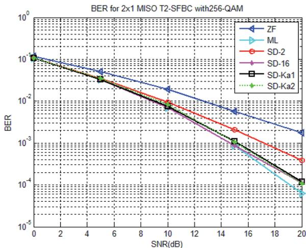
Fig. 3. BER Performance for AKBSD (SD-Ka1, Ka2 legends) versus ZF, ML and different K-SD.
