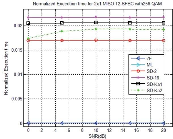
Fig. 4. Complexity in terms of normalized execution time (to ML time) for AKBSD (SD-Ka1, Ka2 legends) versus ZF and different K-SD decoding methods.
